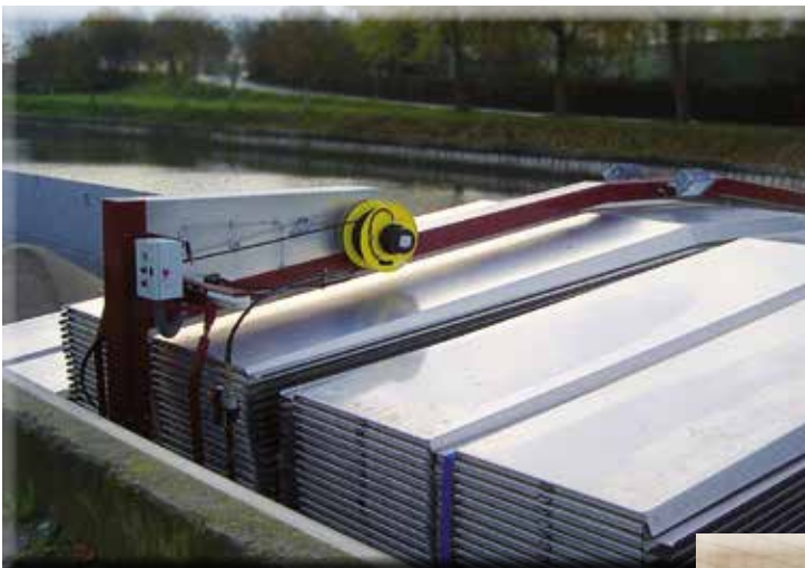
AV28 cable reel for feeding and controlling of a hatch crane on a freight ship
